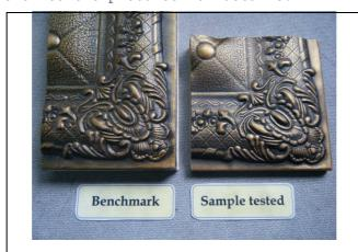
Part showed slight color change. There was no other visible surface damage. After 500 hours test, Gray Scale=4.
