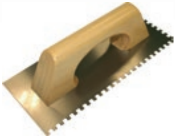
XLIGHT TROWEL 280mm. (10X10mm/ 6X6mm/ 3X3mm) The type of trowel will depend on the thickness of the adhesive coat and this in turn will depend on the type of substrate. The more even the substrate is, the less thick the adhesive coat needs to be.
