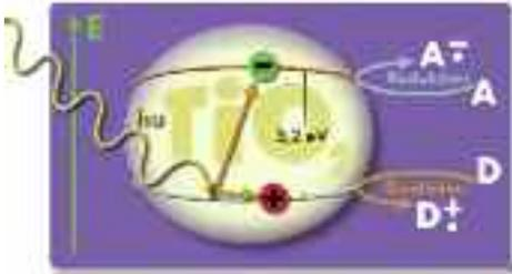
This type of a pigment is now blended into paint formulas which use the chemical reaction that now is accelerated by photocatalysis.
